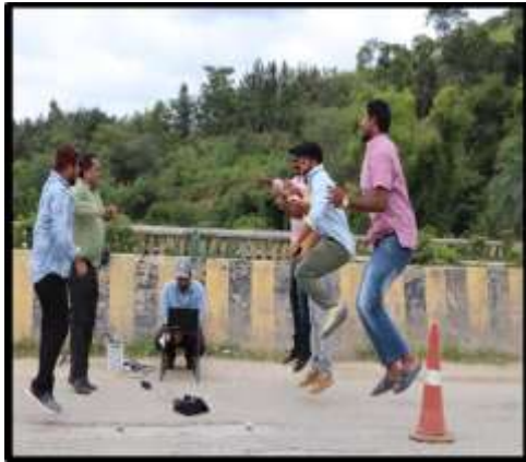
Figure 6. Synchronized jumping test
