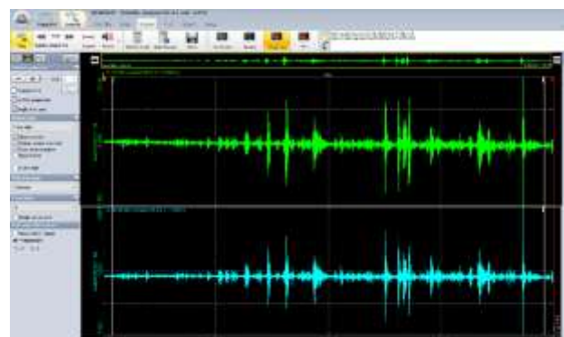
Figure 3. Raw acceleration signals recorded from the bridge using the DEWE-43 data acquisition system
