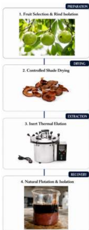
Figure 2. Thermal extraction of Garcinia cambogia rind oil
