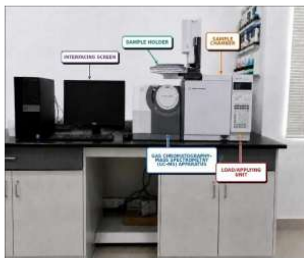
Figure 3. GC–MS system used for chemical characterization
