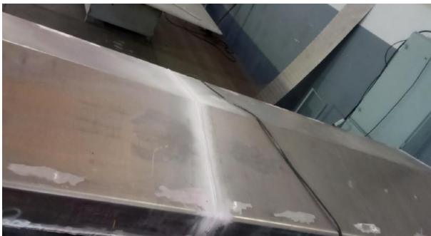
Figure 6. Liquid penetrant testing on fuel tank weld bead
