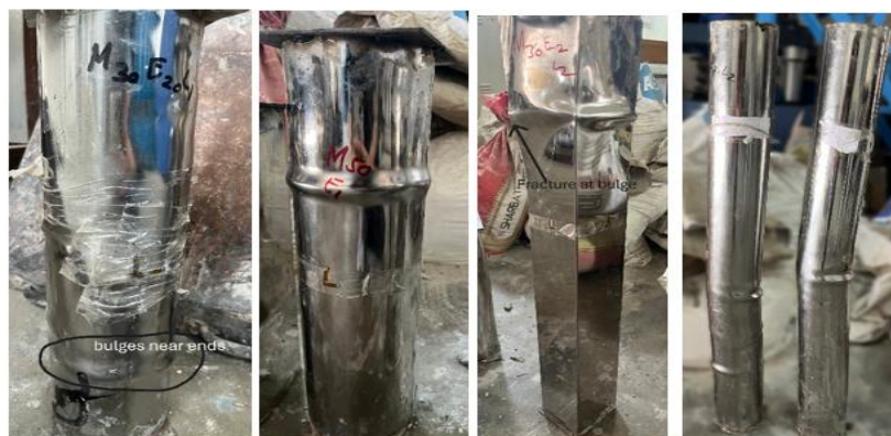
Figure 12. Demonstration of failure modes of various tested samples
