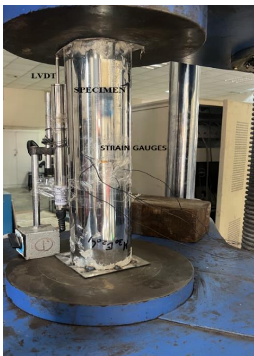
Figure 3. Depiction of experimental setup for axial compression testing of ECFSSST columns
