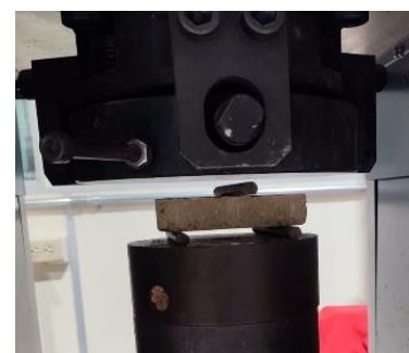
Figure 2. (b) Joist specimen
