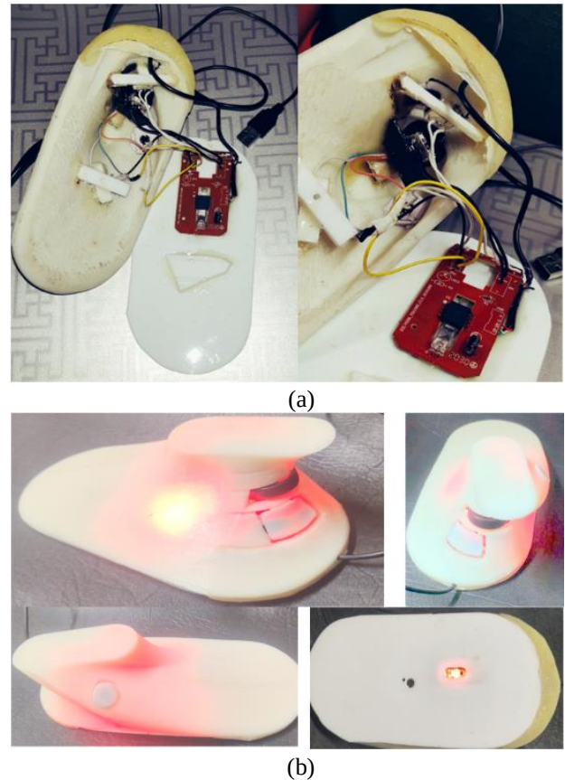
Figure 3. Fabricated mouse based on survey result (a) Arrangement of circuits (b) Functional condition
