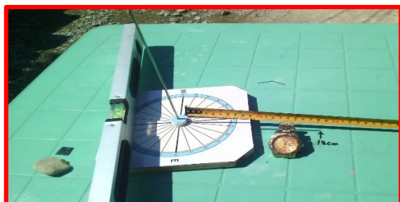
Figure 23. Shadow technique for measuring angle of elevation of the sun Dated February 07, 2023 @ 1:00PM
