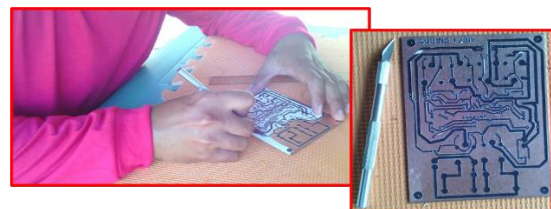
Figure 10. Removing the unused area of the layout
