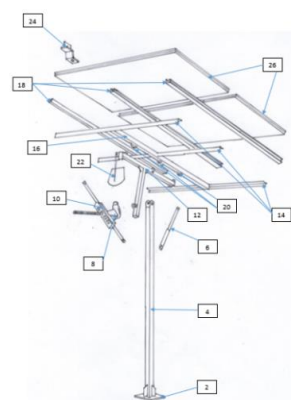
Figure 4. Exploded View of the Solar Tracker Mechanism
