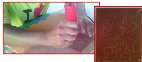
Figure 12. PCB Boring Process
