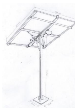
Figure 3. Isometric Drawing of the Solar Tracker Mechanism
