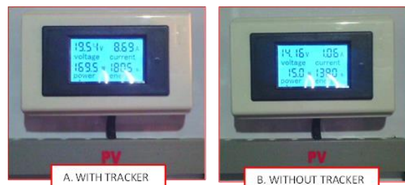
Figure 17. Power Generation of the PV Module at 5PM (With Tracker vs Without Tracker)
