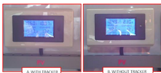
Figure 15. Power Generation of the PV Module at 8AM (With Tracker vs Without Tracker)
