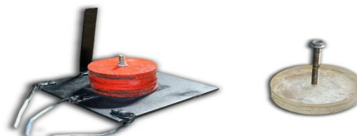
Figure 6. Fixing technique for the load above the foundation
