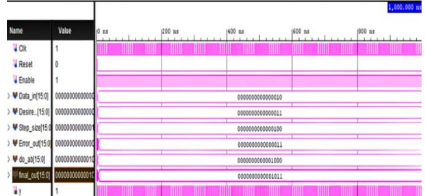
Figure 6. Simulation waveform of LMS Adaptive filters using ROBA multiplier
