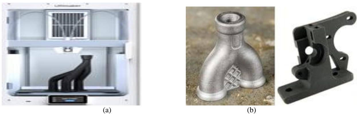
Figure 4. (a) Professional 3D printer UltiMaker S7; (b) End-use parts made with the professional 3D printer UltiMaker S7
