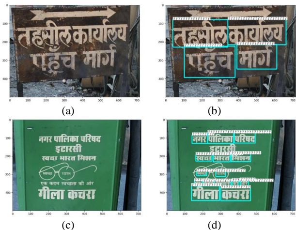
Figure 2. Text localization accuracy (a) shows a standardized image of vpdDataset before training (b) shows scene image localized text by the proposed model (c) depicts another standardized image of vpdDataset before training and (d) presents scene image localized by the proposed model
