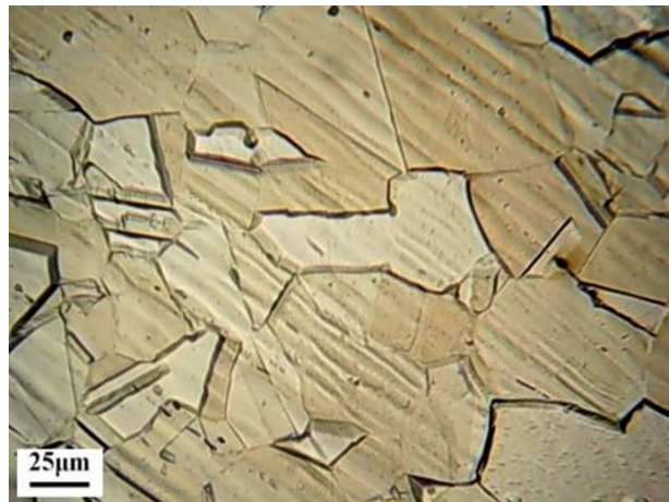
Figure 9. Microstructure of 304LN-SS after sample failure at HT (573K) and 1.1% strain amplitude
