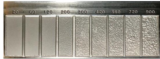
Figure 5. AFS C-9 Micro finish comparator
