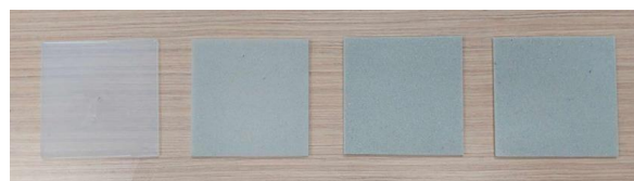
Figure 4. Cured silicone rubber specimens S0, S5, S10 and S15 (from left to right)
