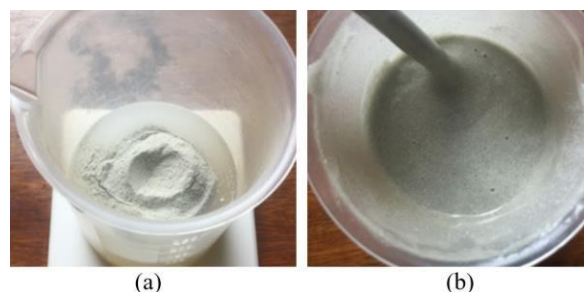
Figure 3. Liquid silicone rubber with quail eggshell filler: (a) before mixing and (b) after mixing
