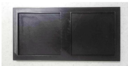
Figure 1. 3-D Printed Mold for Specimen Preparation
