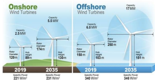
Figure 5. The expected rise in the size of land-based and offshore wind turbines (m: meters; W: watts). National Renewable Energy Laboratory (NREL) graphic by John Frenzl
