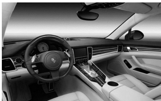
Figure 8. Equipment elements and partially limited visibility from the front pillar
