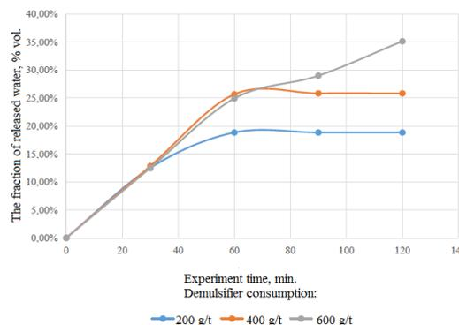
**Figure 2.** Efficiency of Dissolvan-4411 demulsifier from Bulla crude oil at 20 °C
