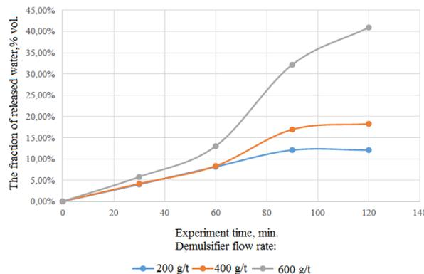
**Figure 1.** Efficiency of Dissolvan-4411 demulsifier from Muradkanly oil at 20 °C
