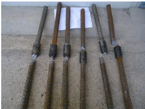
Figure 31. Broken 6 new samples from pier P1, bar \phi 32 , coupler type C
