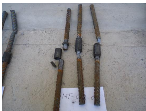
Figure 29. Broken samples from pier P1, bar \varphi 32, coupler type C
