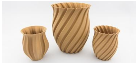
Figure 4. Parts made of Wood PLA
