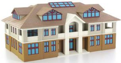
Figure 5. A model made of sandstone with a 3D printer
