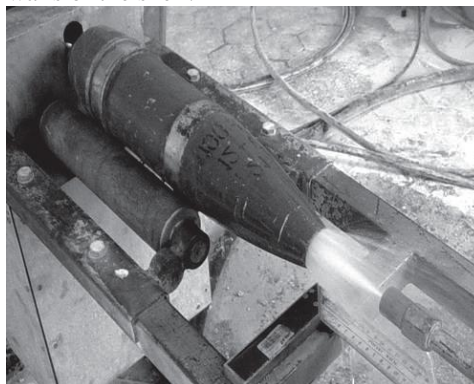
Figure 3. Application WJW of projectile delaboration process
