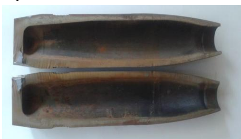
Figure 2. Application AWJ technology in the process of shellcutting
