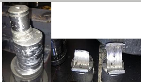
Figure 2. Damage due to wear of the crankshaft and sliding bearing
