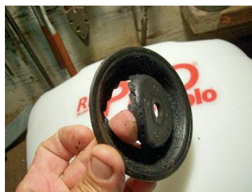
Figure 3. Rupture of the oil diaphragm
