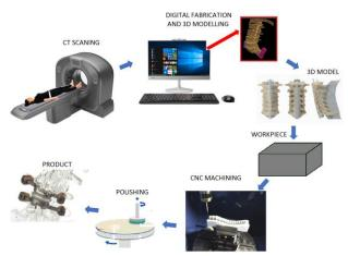
Figure 3. Vertebra manufacturing process based on CT scan images
