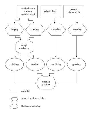
Figure 2. Manufacturing process of hip joint
