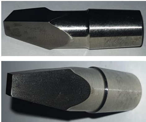
Figure 6. Taper and trapezoidal junctions of femoral neck adapters in CoCr (a) and Ti6Al4V (b) after 2450000 fretting cycles
