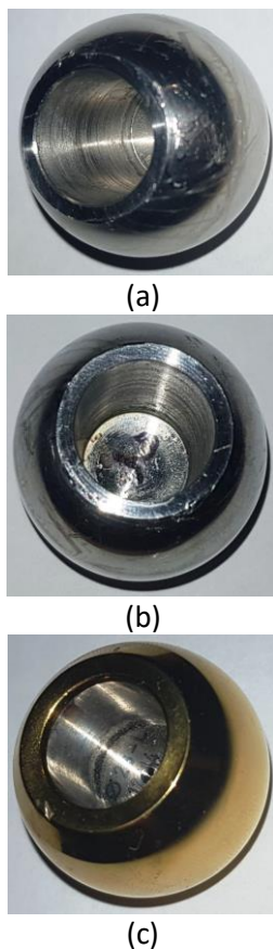
Figure 7. The fretting and corrosion wear of the inner taper of the femoral heads made of CoCr (a), Ti6Al4V (b) and ceramics (c) after 2450000 fretting cycles
