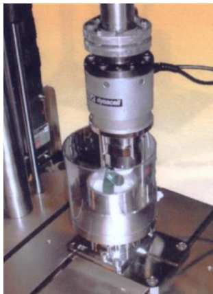
Figure 1. Instron® fatigue testing device of total hip prosthesis
