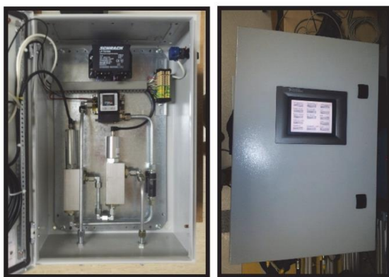
Figure 2. Industrial on-line oil condition monitoring system
