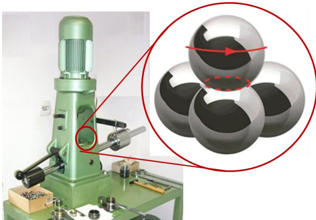
Figure 2. Principle of welding-load and wear-diameter measurement
