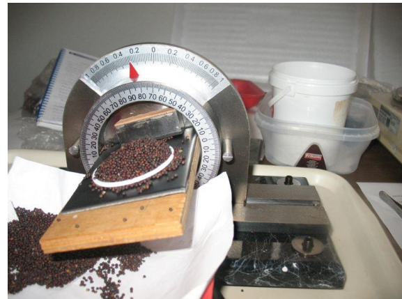
Figure 1. Friction coefficient measuring device Tribometer 1
