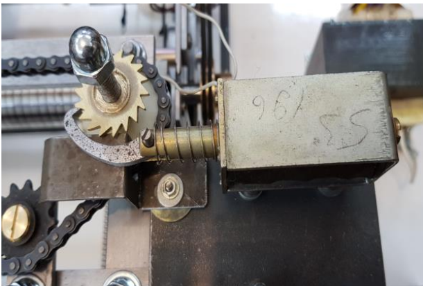
Figure 10. Mechanical transmission system for cutting tool operation
