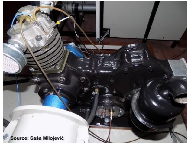
Figure 12. Photograph of the experimental reciprocating air compressor
