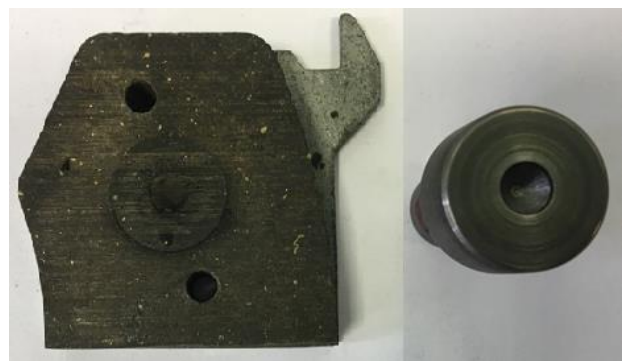
Figure 7. C/SiC (left) and Steel C22 (right) samples after the last experiment
