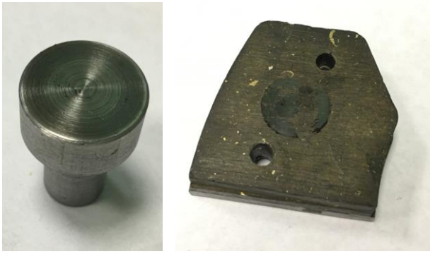
Figure 3. Steel C22 (left) and C/SiC (right) samples after the second experiment
