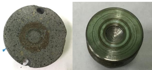
Figure 1. C/SiC (left) and 37Cr4 (right) samples after the first experiment
