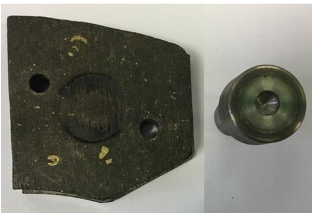
Figure 5. C/SiC (left) and Steel 37Cr4 (right) samples after the third experiment
