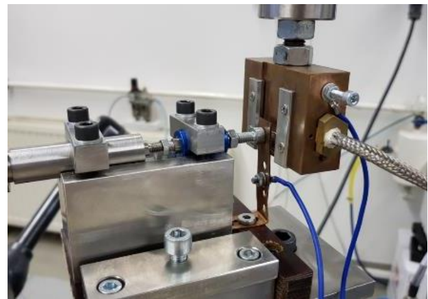
Figure 3. E10000 electrodynamic test equipment with the developed fretting test holders
