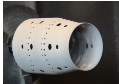
Figure 12. Burning chamber after coating
