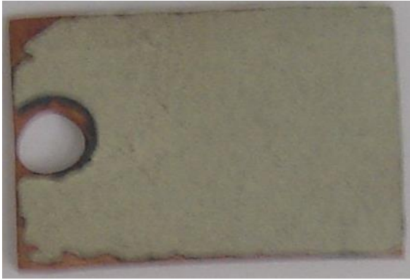
Figure 3. Specimen C9 - NiCrAlY/Al 2 O 3 + ZrO 2 Y 2 O 3 for aircraft industry after being tested at 800°C
