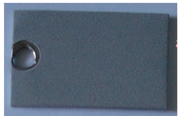
Figure 2. Specimen for aircraft industry before being tested – C9 - \text{NiCrAlY/Al}_2\text{O}_3\text{ + ZrO}_2\text{Y}_2\text{O}_3
