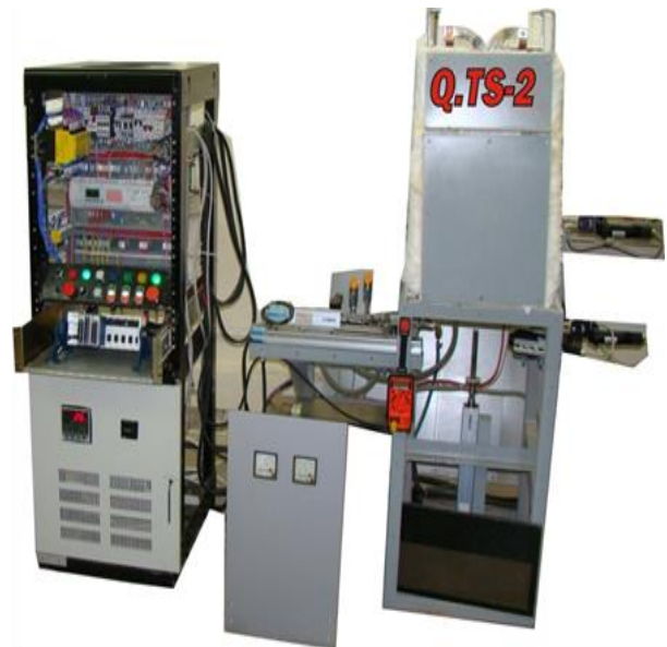
Figure 6. Quick thermal shock installation – Patent number 127339
