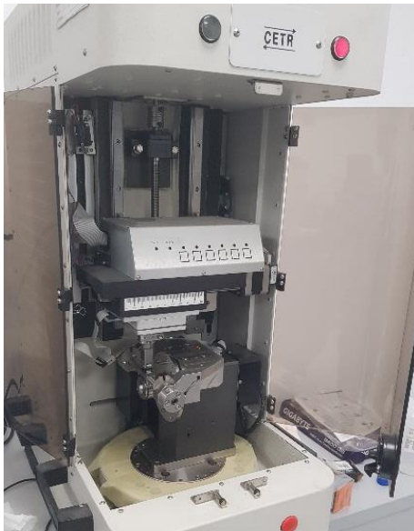
Figure 8. Universal tribometer CETR-UMT-3 Bruker bloc on ring module
