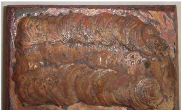
Figure 5. Specimen for metallurgical industry before being tested - Cu/Casto TIG (cooper and silver alloy x3)
