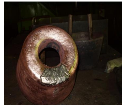
Figure 14. Tuyere after coating
