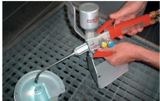
Figure 1. Device for manual gas fuel deposition (Reproduced by permission of Castolin Eutectic [6])
