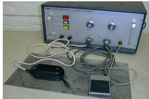
Figure 2. Device for Manual electrical discharge deposition with vibrating electrode “Harddege” - England, USA
