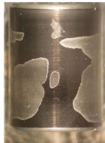
Figure 6. Delamination failure of ta-C DLC coating on 100Cr6.
