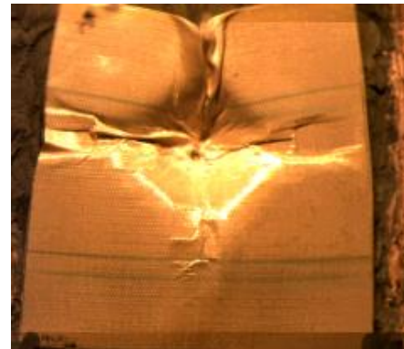
Figure 12. layers of LFT SB1, 9 mm FMJ, 400 m/s, fast camera image [26]
