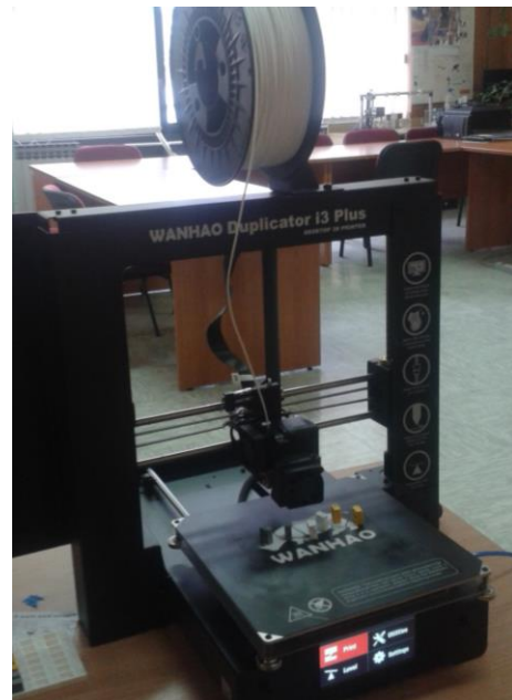
Figure 1. WANHAO 3D printer
