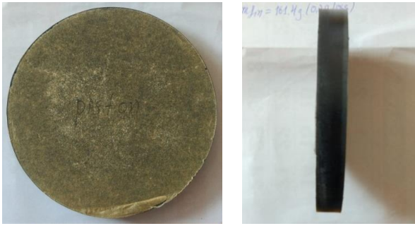
Figure 2. Picture of a disk blank with a diameter of 124 mm from composite UHMWPE-0.75CNTs: a) face, b) side
