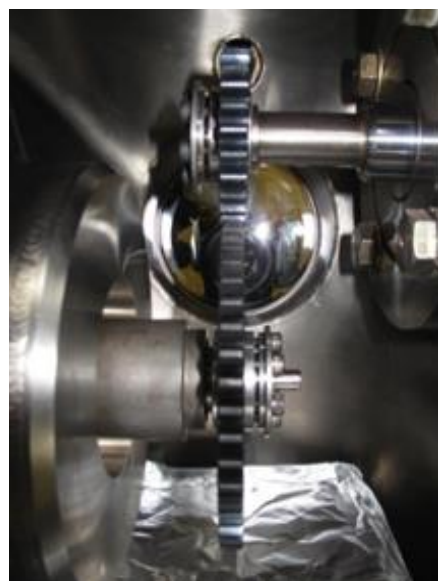
Figure 3. Test gears: (a) Just prior to testing, (b) Installed in rig just prior to closing test chamber.
