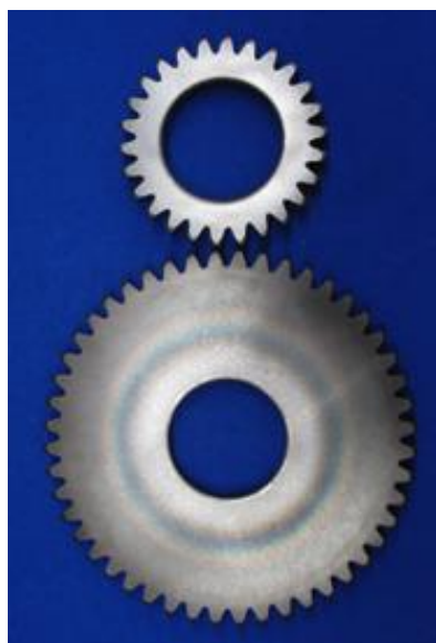
Figure 3. Test gears: (a) Just prior to testing, (b) Installed in rig just prior to closing test chamber.
